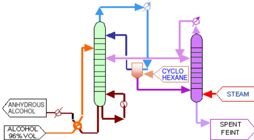
**PFD OF AZEOTROPIC DISTILLATION PROCESS**
